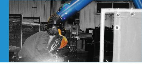
Avani's SPC-1000 is a user friendly versatile portable fume extraction system. The four stage filtration and optional filtration configurations offer a highly efficient and effective clean air solution. Single phase 120 volt power, casters and vertical compact design make the SPC-1000 the perfect choice for point of origin fume extraction at any location in the plant or shop.
